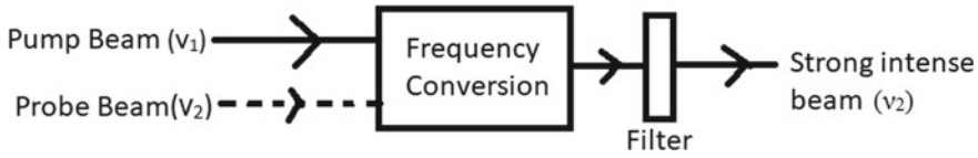
Fig. 1 Frequency conversion from pump to probe by XGM process of SOA
