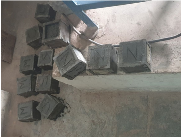
Fig. 3 Geopolymer cube casting
