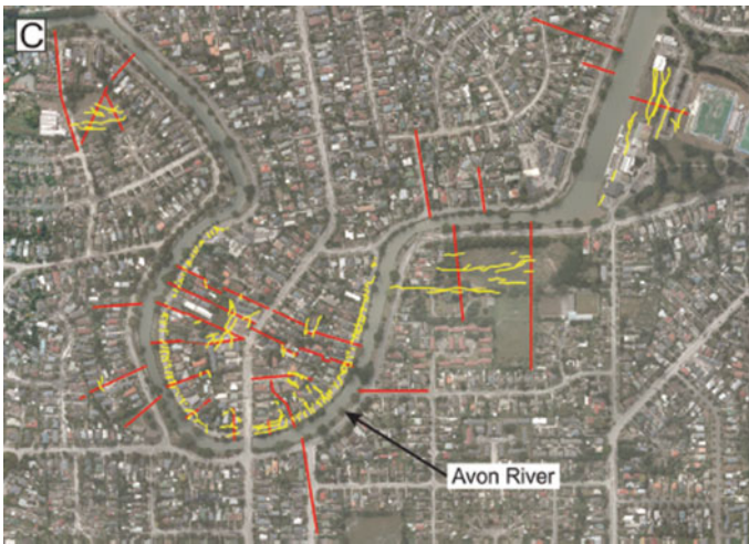
Fig. 5 Induced Lateral spreading effect from Avon River into the CBD Source (Cubrinovski et al. 2012b)
