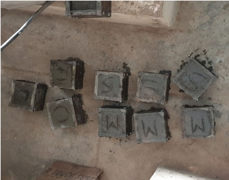
Fig. 4 Mortar cube casting
