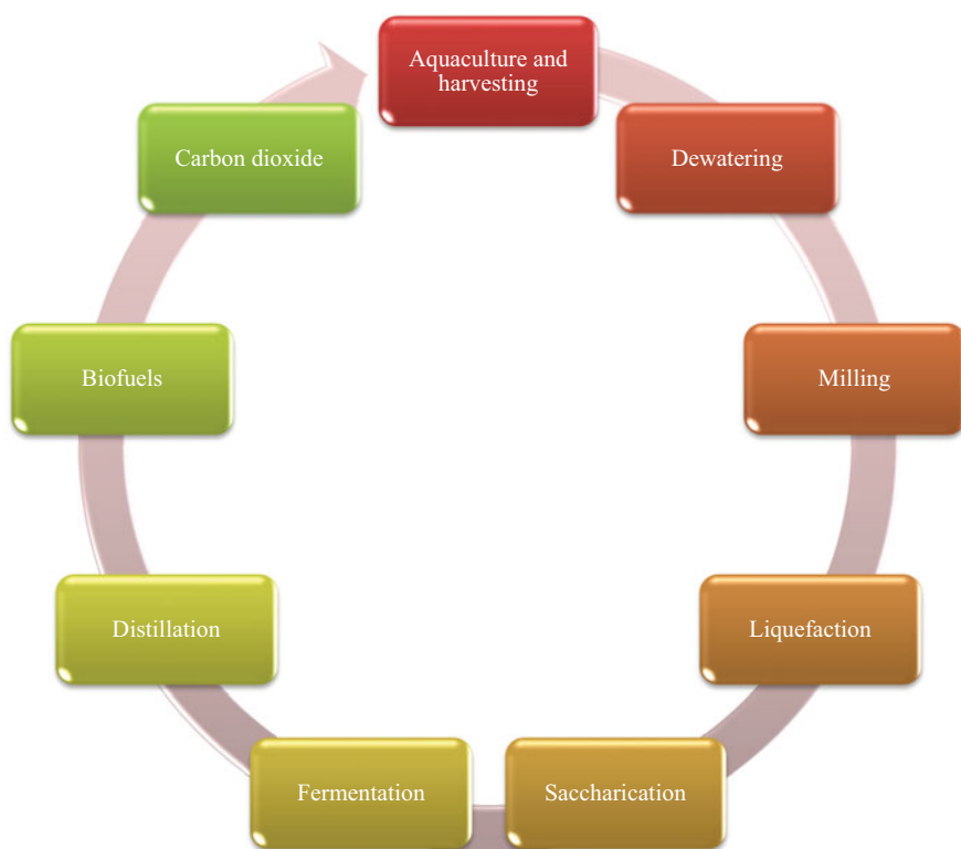
Fig. 3.9 Production of bioethanol from algal biomass through fermentation process
