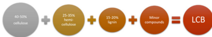
Fig. 4.2 Chemical composition of lignocellulosic biomass (LCB)
