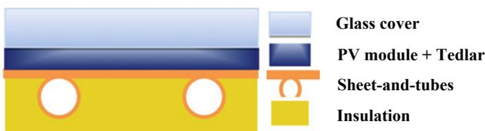
**Fig. 1** PV/T “sheet & tubes” system design
