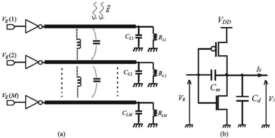
Fig. 2 a  $M$ -interconnects coupled with drivers and loads. b CMOS inverter model
