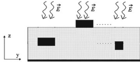
Consider  $M$  imperfect interconnect lines immersed in an incident field, as shown in Fig. 1, modeled by the following system of coupled partial differential equations (Telegrapher’s equations) [10, 11]:
