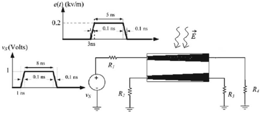
Fig. 5 Schematic of two nonuniform interconnect lines in the presence of an external field  $\vec{E}$
