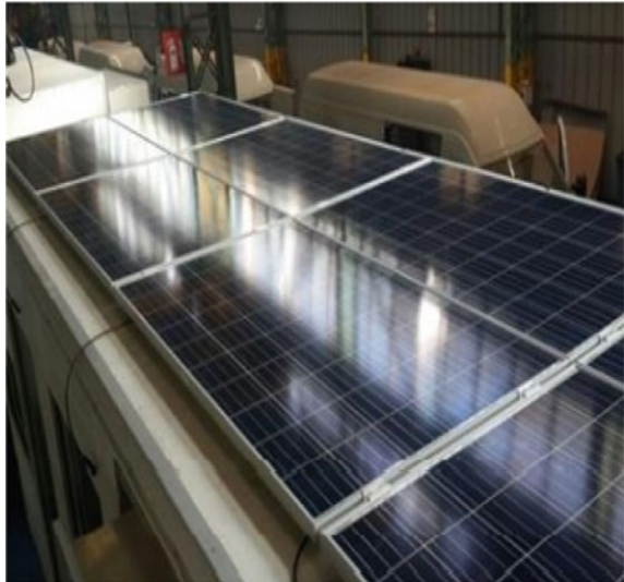
Fig. 2 Solar photovoltaic array mounted on the roof of the truck
