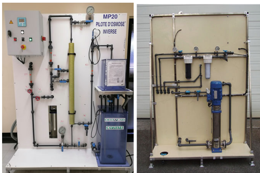
Fig. 3 Front and rear face of the MP20 RO pilot
