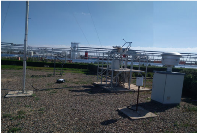
Fig. 1 Soiling station equipped with TraCS and meteorological instrument measurement
