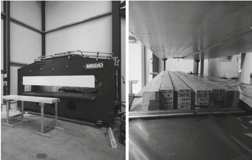
Fig. 6 TimberPress X 300 (left) for pressing the GLT. Alignment of the GLT beams in the press, with lateral restraint between the beams (right)
