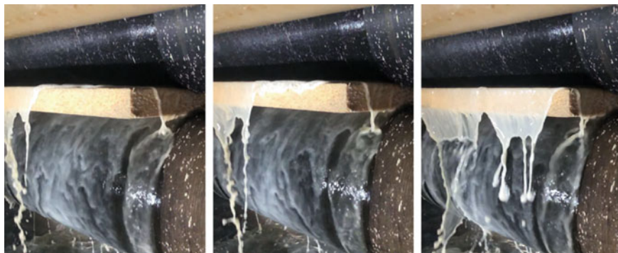
Fig. 4 Compression of an intermediate board with roller press
