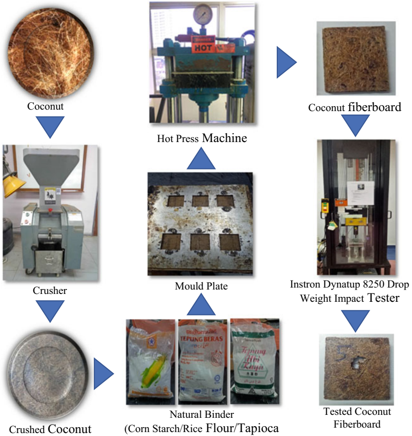
Fig. 1 Fabrication process of coconut fiberboard (CFB)
