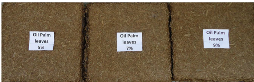
Fig. 5 Performance of OPL's particleboard bonded by UF resin with different amounts of hardeners, namely 5%, 7% and 9% (from Ref. [38])
