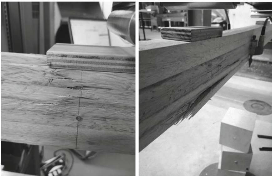
Fig. 7 Typical fracture patterns; left: in compression below the load inducing area and in the area of the supports; right: in tension on a reverse loaded beam
