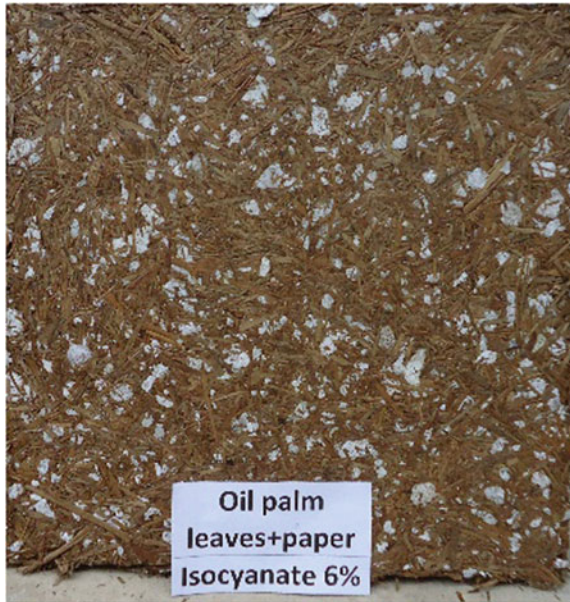
Fig. 9 Typical performance of sound insulation board made of OPL and recycle paper (from Ref. [50])
