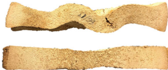
Fig. 1 Typical cell collapse in oil palm wood after improper kiln drying
