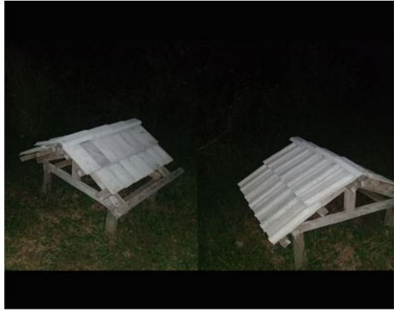
Fig. 1 Flat and corrugated roofing tiles at 720 days of weathering
