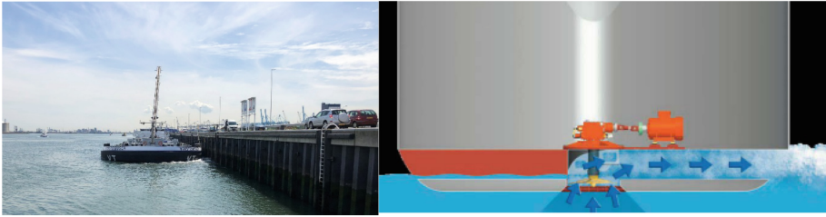
Fig. 1. Measurement location with the Vorstenbosch (left); Schematic representation of a 4-channel bow thruster, illustrating the working principle of the system (Right, source: vethpropulsion.com).
