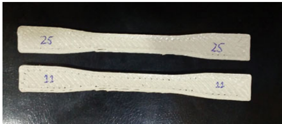
Fig. 5 Tensile specimens printed with ABS
