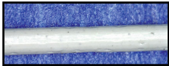
Fig. 3 Microscopic image of ABS throughput
