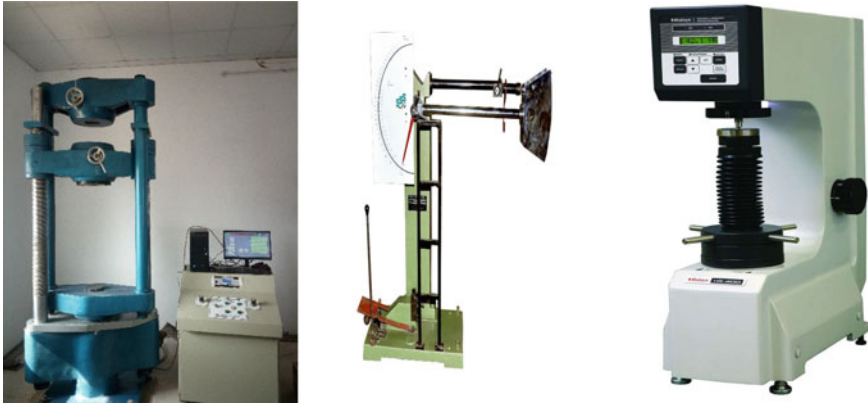
Fig. 2 Various mechanical testing machines—universal testing machine, Izod-Charpy machine, and Rockwell hardness testing machine
