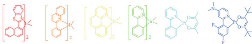
Fig. 3.9 Chemical structures of some typical wavelength-tunable metal complexes. Adapted from Ref. [2]
