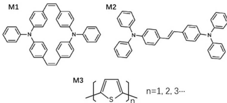
Fig. 1.24 Molecule structures of macrocycle (M1) and linear chain (M2) with triphenylamine units and oligothiophene nT (M3)
