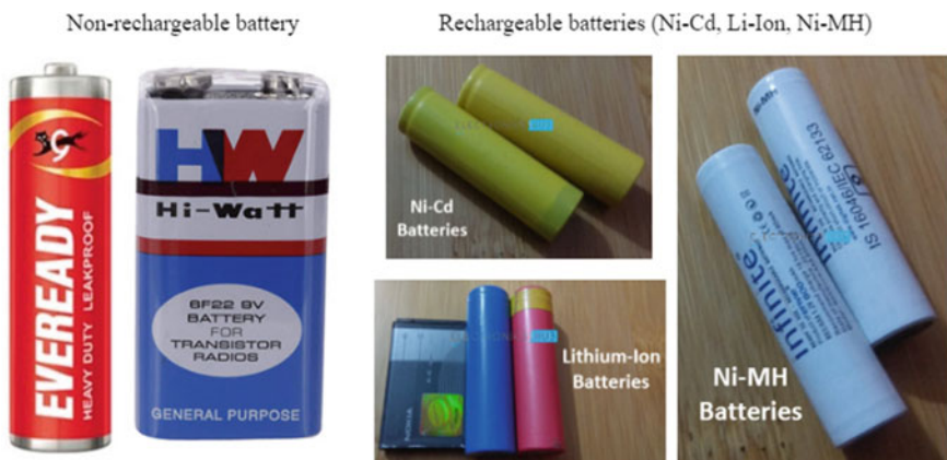
Fig. 2 Representation of rechargeable and non-rechargeable battery
