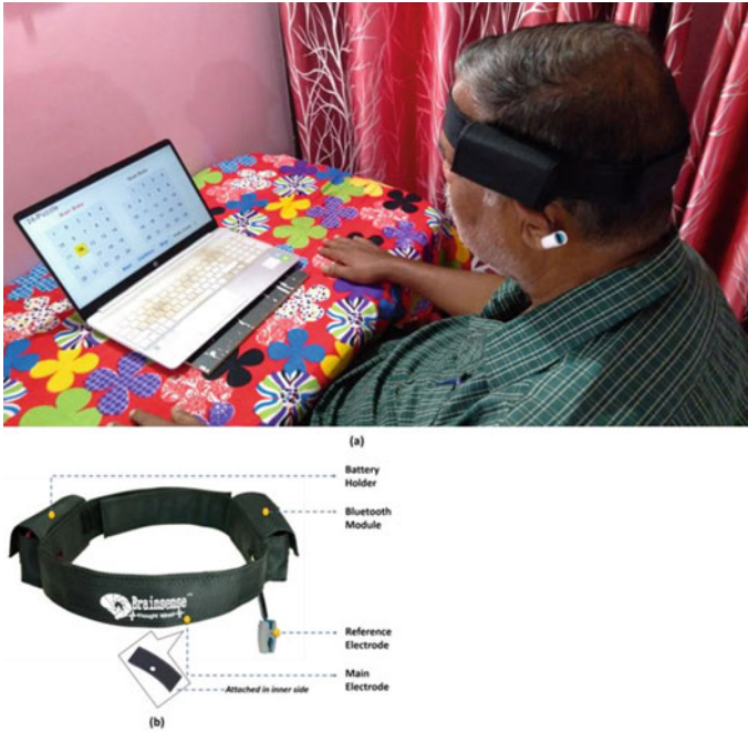
Fig. 29.1 Mapping of 10–20 electrode placement with electrodes of Brainsense BCI headset. a Subject (64 years age) wears single-channel BCI headset (Brainsense) and interacts with the GUI-based puzzle b Components of Brainsense
