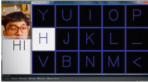
Fig. 43.7 Result through live video-stream of eye gaze detection in virtual keyboard
