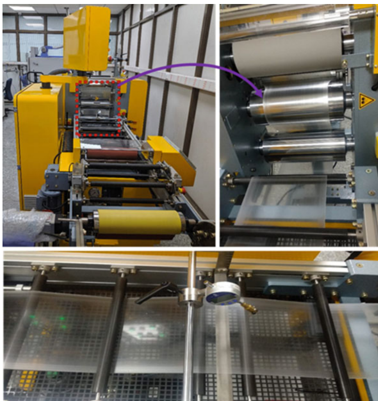
Fig. 1 Different stages of aliphatic and aromatic TPU film preparation by using single screw extruder connected with film casting unit
