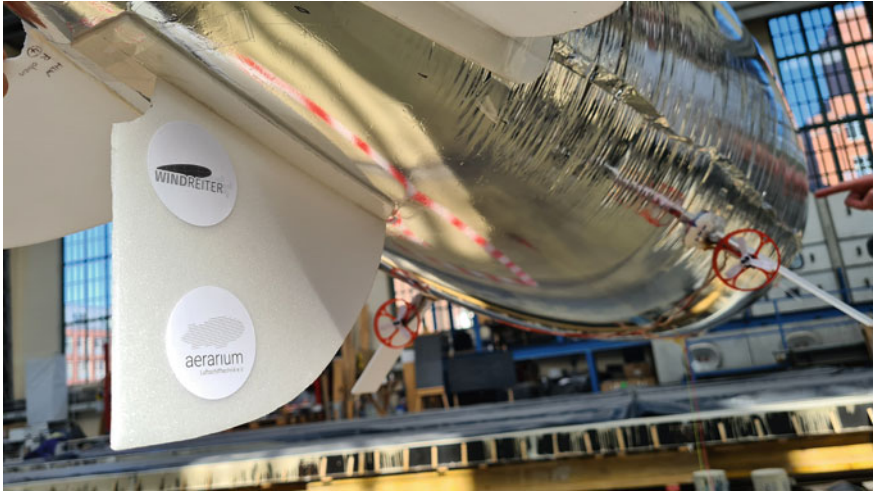
Fig. 7 Close-up of the airship model used. The pig-leg configuration of the propulsion system allows dynamic positioning of the airship
