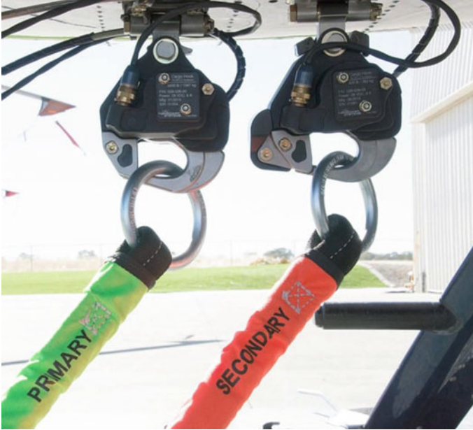
Fig. 2 Onboard Systems' MD500 Dual Cargo Hook kit with Y-rope [8]
