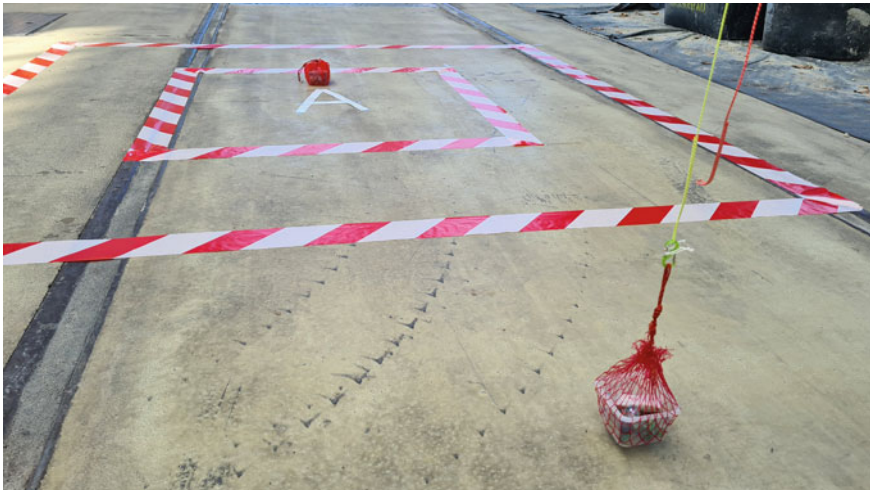
Fig. 8 The landing site is indicated by an ‘A’ for airship and marked with a two by two meter square and a smaller one by one meter square allowing for a rating of maneuverability. Both cargo loads, one attached to the airships sling and one at the loading site, are equal in weight
