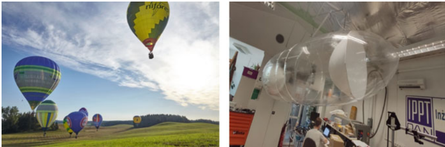
Fig. 2 a Balloon SKYLAB and b mini-model CANDY with two ballonets
