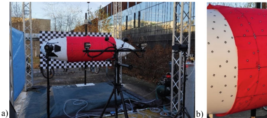
Fig. 4 Experimental set-up: a experimental object and set-up of cameras and b optical markers on the surface
