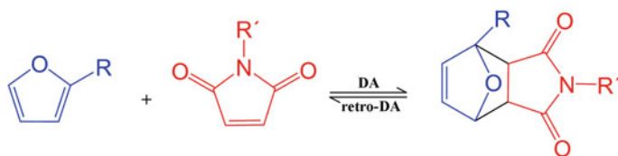
Fig. 2 DA and retro-DA reactions between maleimide (M) and furan (F). Reprinted with permission from [31]
