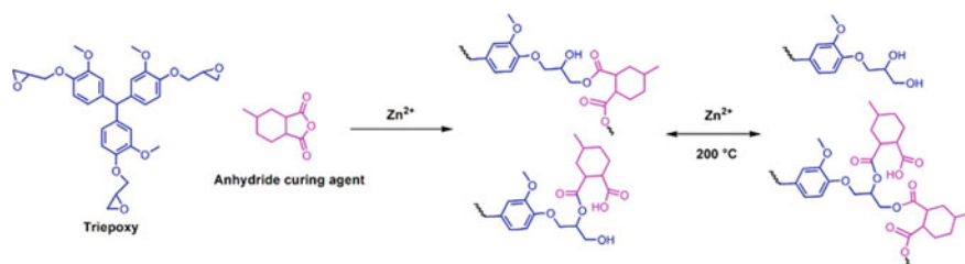
Scheme 4 TEP and anhydride curing reaction and illustration of dynamic transesterification reactions (TERs) in a cross-linked network structure (Reprinted (adapted) with permission from [27]. Copyright (2018) American Chemical Society)
