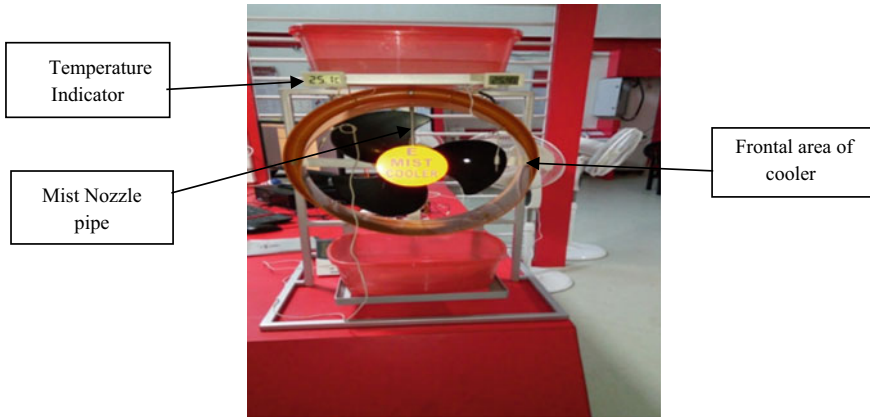
Fig. 5 Experimental set-up of evaporative cooler
