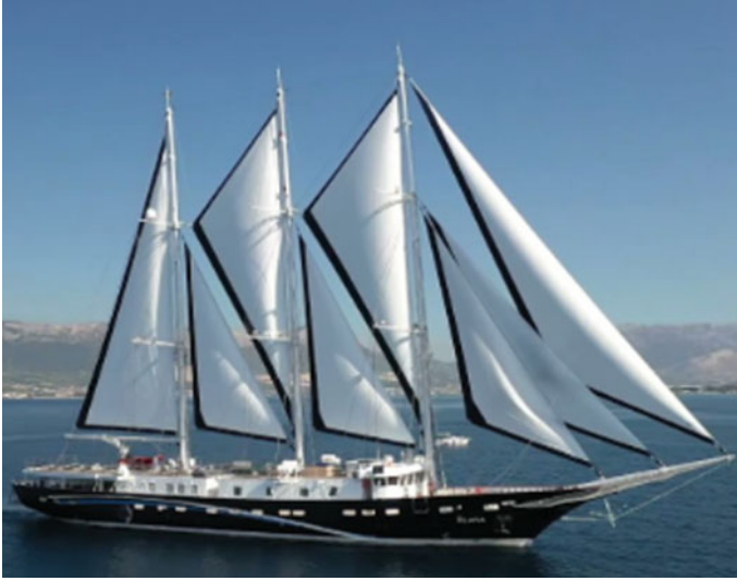
Fig. 7 Three mast schooner passenger sailing ship Klara is 64 m long, 10 m wide, with the height of 5.35 m up to the main deck. Gross Tonnage: 497 t and max speed above 11 knots 2 \times ICE 368 kW, 8 sails with a total area of 845 m 2 , and two 150 kW diesel generators
