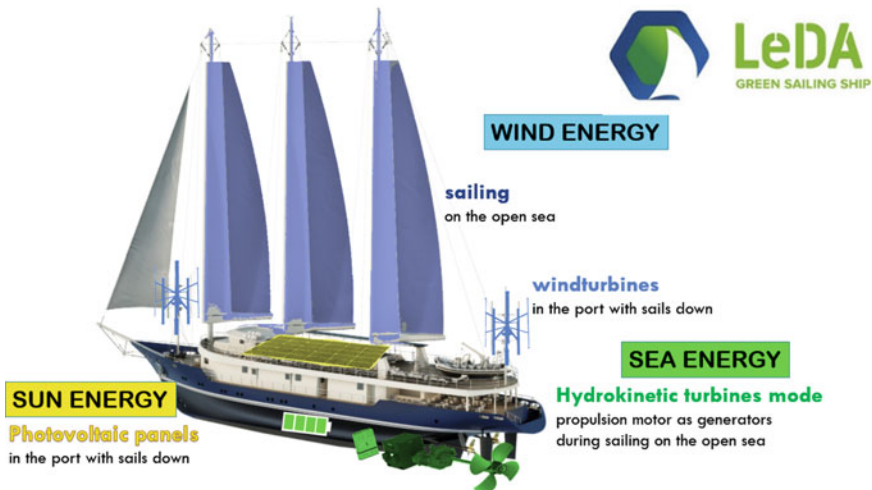
Fig. 14 Hybrid energy recuperation from different RES: wind energy during sailing on open sea (movement of ship, recuperation of kinetic energy via hydrokinetic turbine mode of ship main propellers), wind energy during anchored time with sails down via small wind turbines, sun energy via photovoltaic panels
