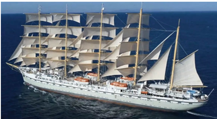
Fig. 6 Golden Horizon—speed 20 knots, length 162 m, weighs 24 tons, 5 masts with 36 cross sails, total area is 6347 m 2 , total energy consumption ~4.2 kWh
