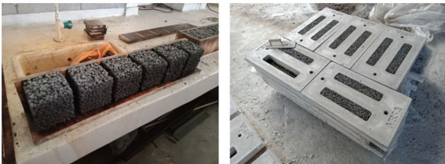
Fig. 1 Samples of cube (left) and drain cover (right) with different sizes of aggregates
