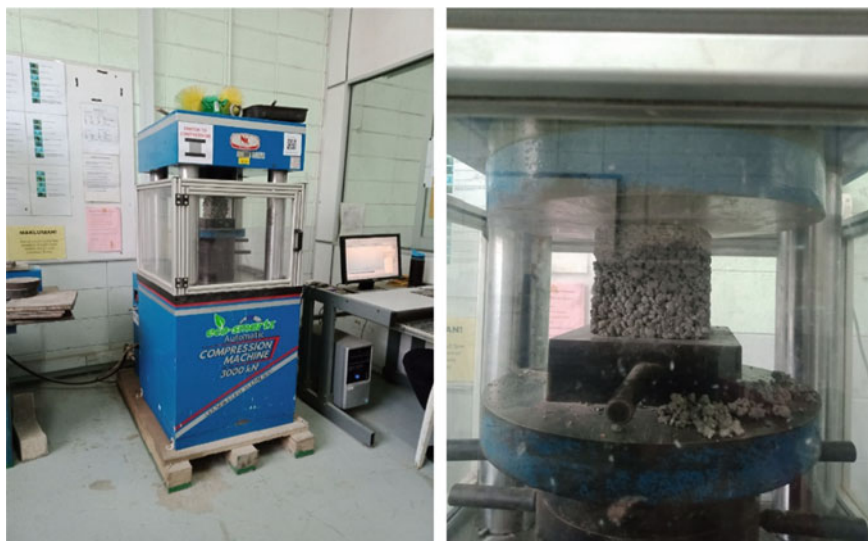
Fig. 3 Compressive strength test for cube samples with different sizes of aggregates
