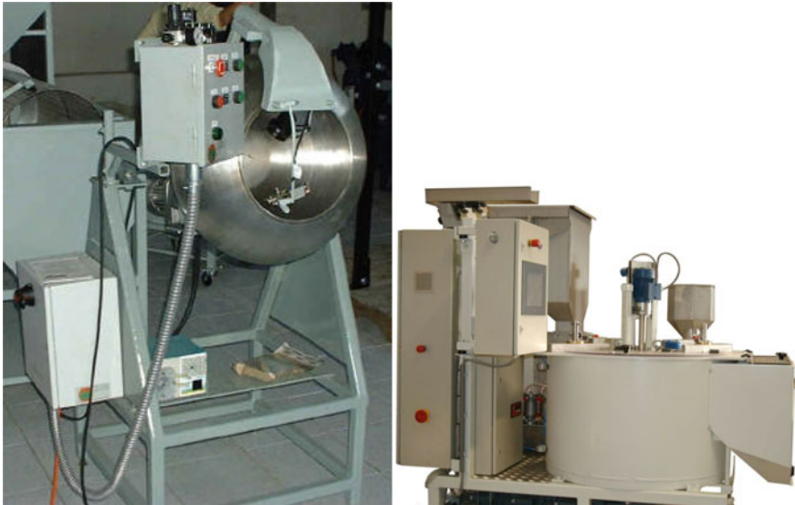
Fig. 12 External views of seed coating/pelleting machine. (Source: http://www.seedpelletingequipment.com/coatingpan.htm )
