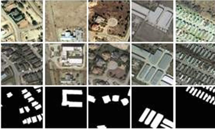
Fig. 5 Chosen samples ( 256 \times 256 ) cropped images from LEVIR-CD. Each column denotes one sample, comprising the image pair (rows 1 and 2) and label (the last row, white representing change and black as no change)
