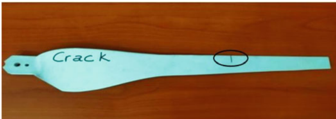
Fig. 5 Blade with crack
