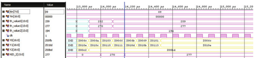
Fig. 13 Simulation waves of directed test verification for 5G NR PSS block
