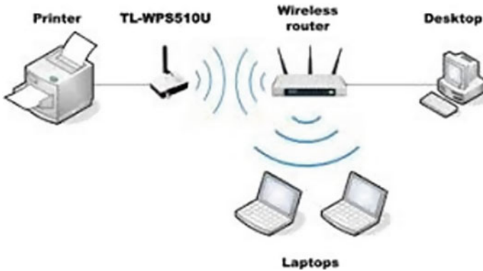
Fig. 2 Infrastructure wireless network
