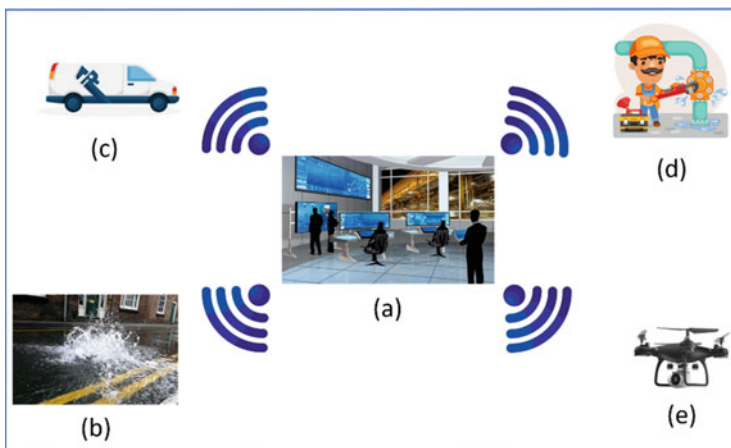
Fig. 1 Control system architecture overview: a SC municipality control centre, b flood water leak, c municipality plumb vehicle, d personnel plumber, and e UAV
