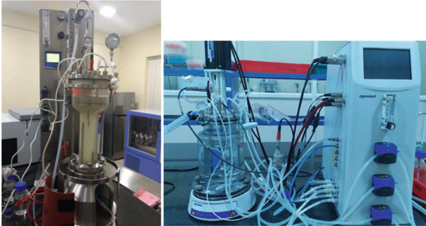
Fig. 19.5 Bubble column and marine impeller bioreactor
