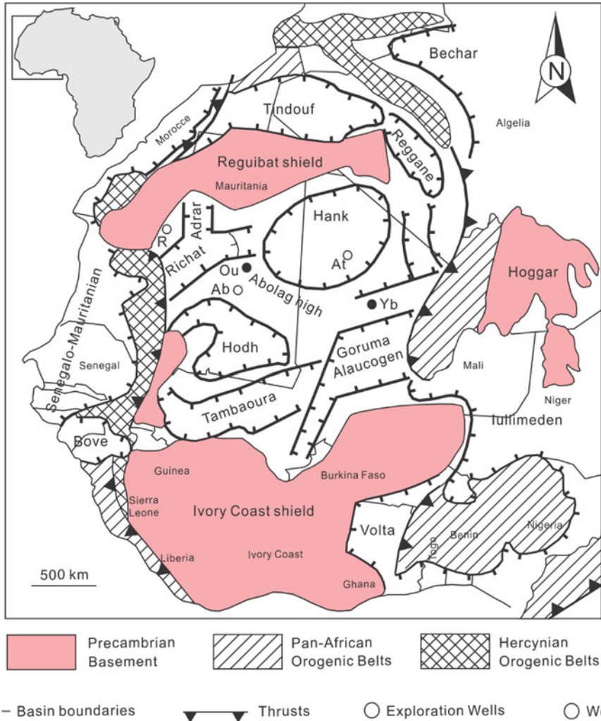
Fig. 11.17 Simplified structural map and oil exploratory well distribution of the Taoudeni Basin (Albert-Villanueva et al. 2016, modified). R. R Well; Ab. Abolag-1 Well; Qu. Quassou-1 Well; At. Atouila-1 Well; Yb. Yarba-1 Well
