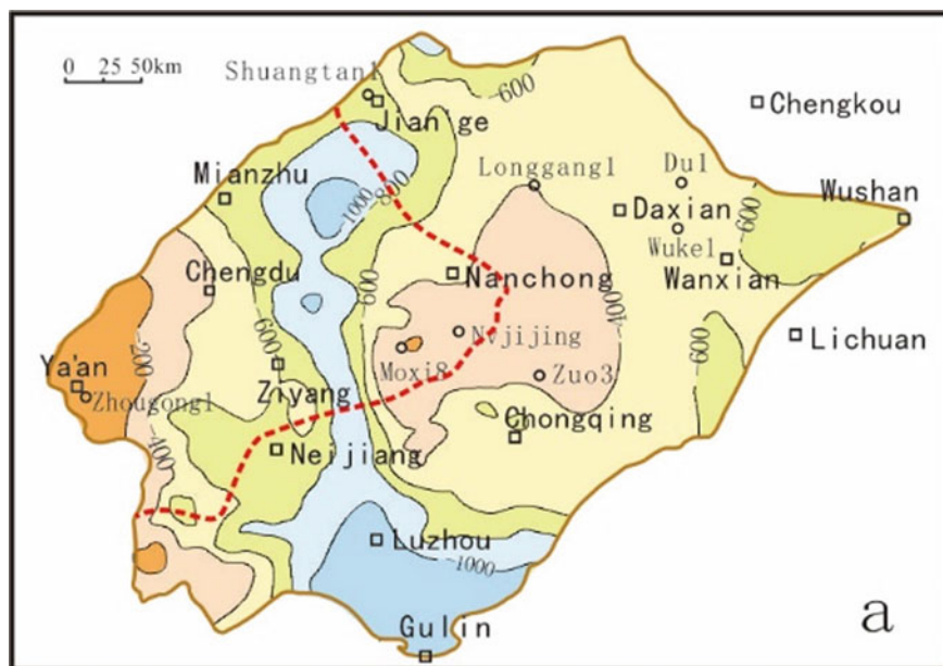
Fig. 14.1 Palaeo-structural contour map of Sinian top surface on Chuanzhong Uplift before the sedimentary period of Longwangmiao Formation ( \epsilon_{11} ) showing the distribution of Deyang-Ziyang Faulted-Sag (in light-blue colour), Moxi-Gaoshiti Anticlines (in light-orange colour) and Weiyuan Anticline (in dark-orange colour). The map range is only limited to current Sichuan Basin
