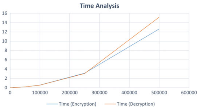
Fig. 5 Graph between the number of characters in the string and time taken to encrypt and decrypt
