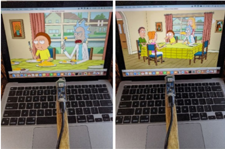
Fig. 20 Sequence of experiments uses gestures as input to a multimedia video player and plays and pauses the video
