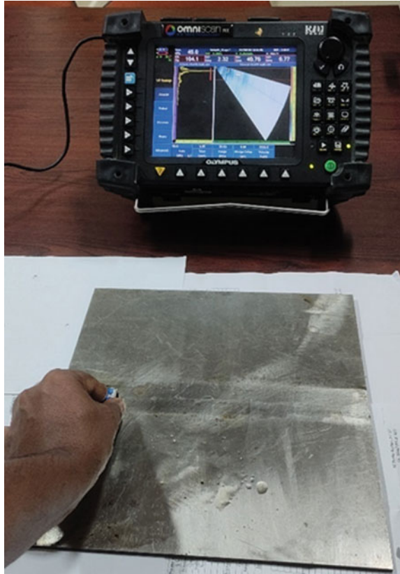
Fig. 5 Scanning of F-notch reference plate
