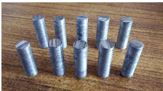
Fig. 1 Cylindrical test sample pins with worn-out surface
