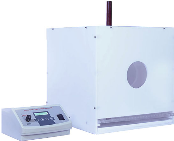
Fig. 6.14 Cook's pole-climbing apparatus
