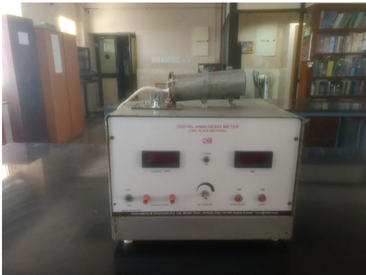
Fig. 6.8 Digital analgesiometer using radiant heat
