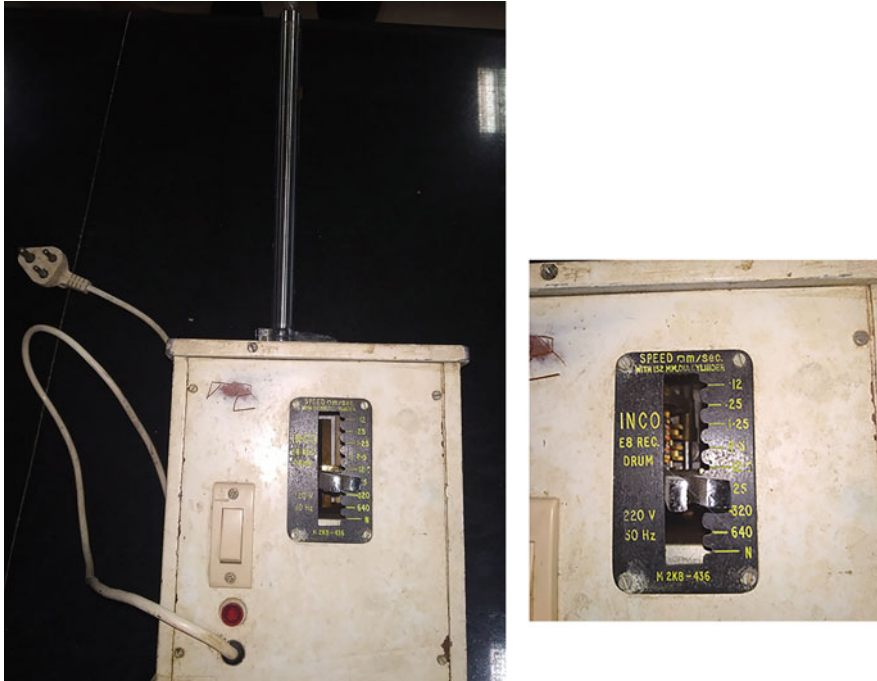
Fig. 6.2 Kymograph with lever for speed adjustments
