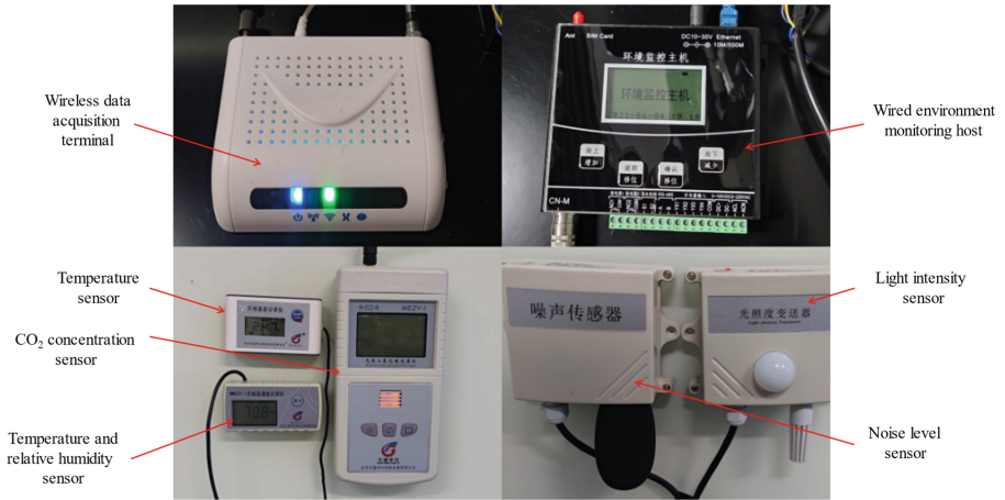
Fig. 1. Hosts for communication and environmental sensors
