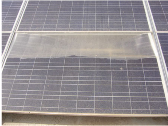
Fig. 7 PV module affected by delamination [6]
