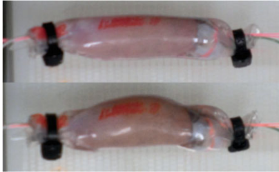
Fig. 10.26 Skeletal muscle tissue actuator surrounded by a silicone membrane. The upper figure indicates natural length. The lower figure shows contraction of the actuator
