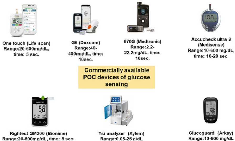
Fig. 5.6 Some commercially available POC devices for invasive glucose sensing: YSI analyzer a trademark of Xylem Inc., its proprietary immobilized enzyme electrodes allowing rapid, accurate measurement in a min., Accu check ultra 2 finger pricker, small and slender device with alternative site testing spacer, Medtronic 670g system enables the personalization of glucose with adjustable target setting as low as 2.2 mmol/L, Dexcom G6 system have slim sensor continuously measures glucose level beneath the skin and sends data wirelessly on a display device. One Touch life scan color sure instantly shows when sugar numbers are in or out of range and syncs data seamlessly with oneTouch reveal mobile app. Glucoguard Arkay has safe eject button and auto coding function for before and after meal results, Rightest GM300 by bionime is safe, convenient with wide LCD screen, and smart accuracy testing within 8 s
