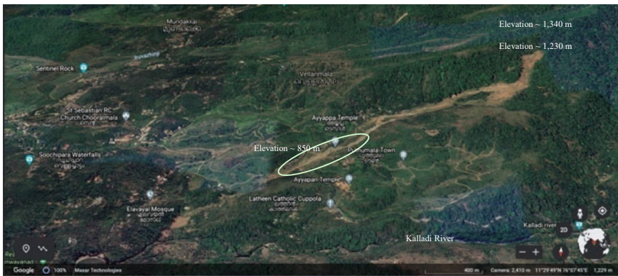
Fig. 3 Google Earth image of the Puthumala landslide site (imagery date: after February 23, 2021); the slide occurred along the course of a stream (Pachakkad-Puthumala thodu) that eventually drained into the Kalladi River flowing north of Puthumala Hill; the flood plain of the stream is circled
