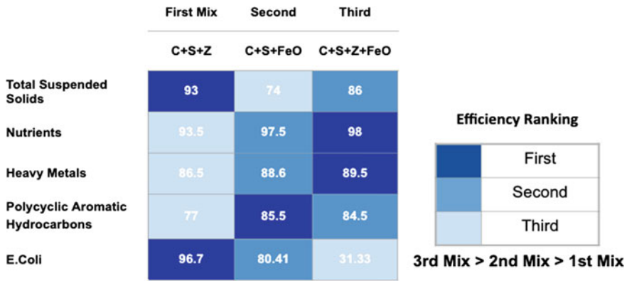
Fig. 1 Ranking of filter media’s contaminant removal efficiencies
