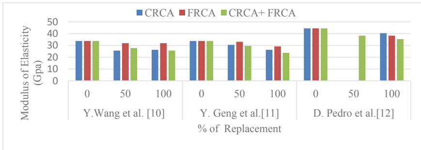
Fig. 6 Elastic modulus of RCA for different literature studies
