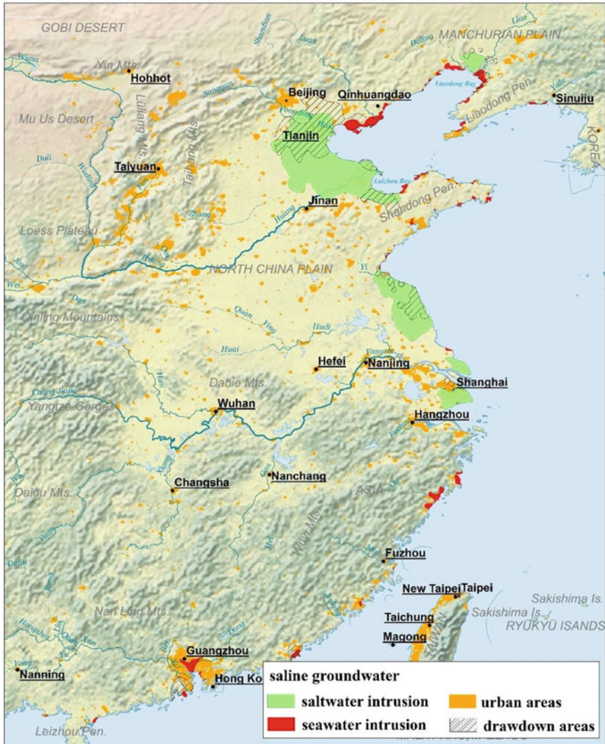
Fig. 5.2 Groundwater drawdown areas and saline groundwater distribution
