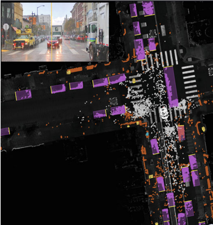
Fig. 1 Onboard Compute perception of surrounding environment around the AV
