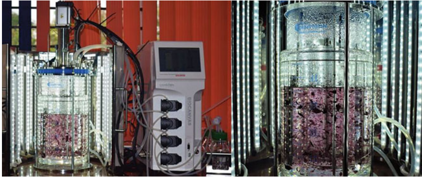
Fig. 3 Closed photobioreactor—capacity: 5 L; light module: LED lamp; max. lux: 20,000 lux; sensor control and recording: pH, DO, temp., foam, and pressure; sparger and gas mode: micro sparger, 2 gas and 4 gas mixers; agitation range: 10–1500 rpm; feeding control system: peristaltic pump control acid, base, foam, and feed; power voltage: 110–220 V, 20.60 Hz, 10 A
