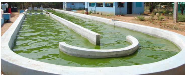
Open Raceway pond cultivation in Department of Microbiology field facility, Bharathidasan University, Tiruchirappalli
