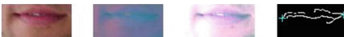
Fig. 5 Lip corners detection: original RGB image, YCbCr representation, fusion of RGB and YCbCr, and lips with edge and corners detection, respectively
