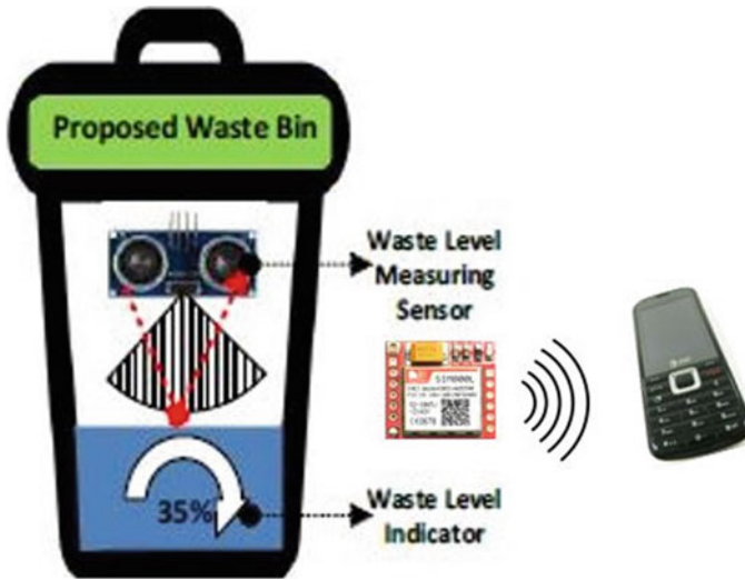
Fig. 4 Bin communication system
