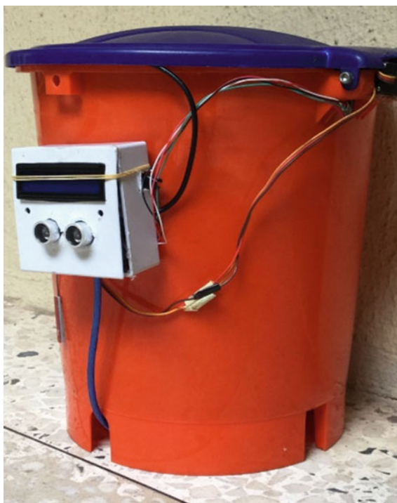
Fig. 5 The designed smart waste bin
