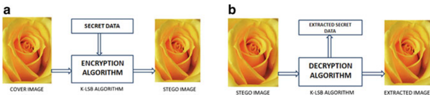
Fig. 2 a Encryption of data inside an image and b extraction of message from Stego image
