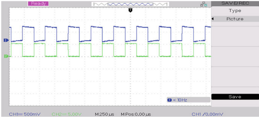
Fig. 12 Switching pulse of multi-input KY boost converter
