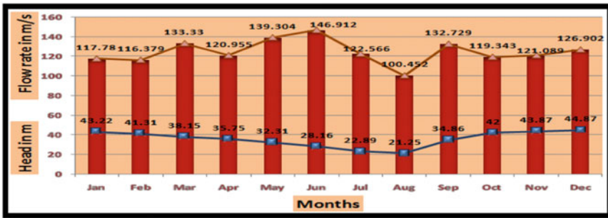
Fig. 3 Monthly average information of head in (m) and water flow rate in (m/s) [9]
