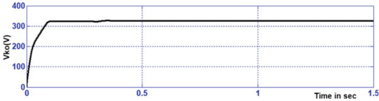
Fig. 3 Voltage across KY boost converter
