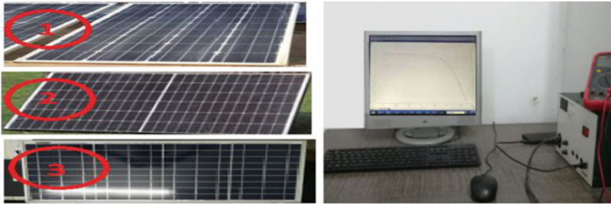
Fig. 2 Experimental setup (left) photovoltaic modules with (1) full-size (2) half-cut and (3) quarter-cut solar cells (right) Indoor experimental setup
