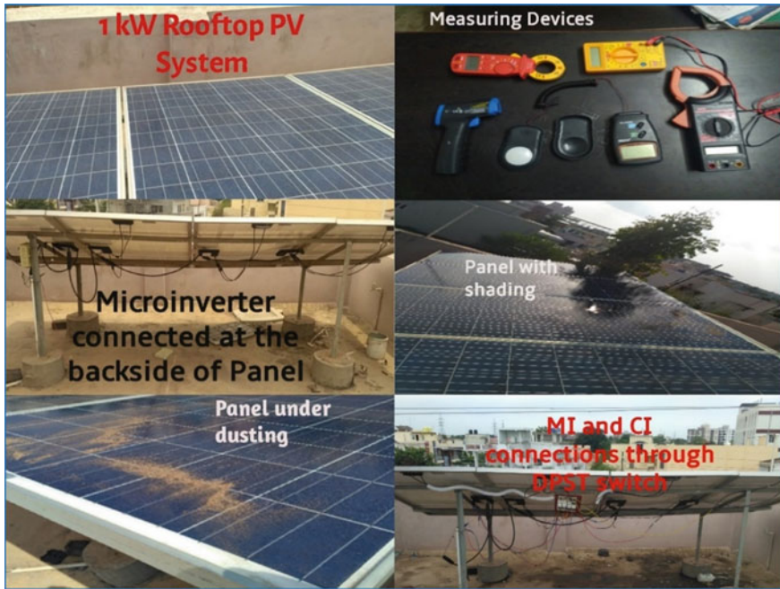
Fig. 3 Experimental setup for CI and MI performance analysis
