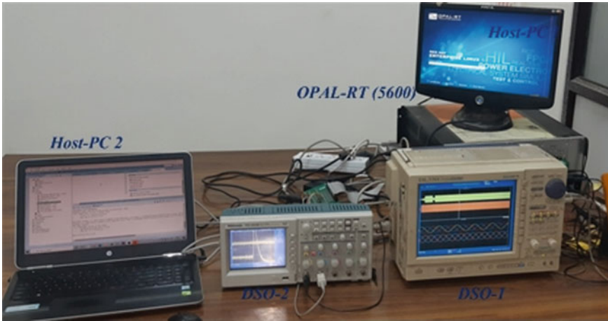
Fig. 12 Real time OPAL-RT experiment setup
