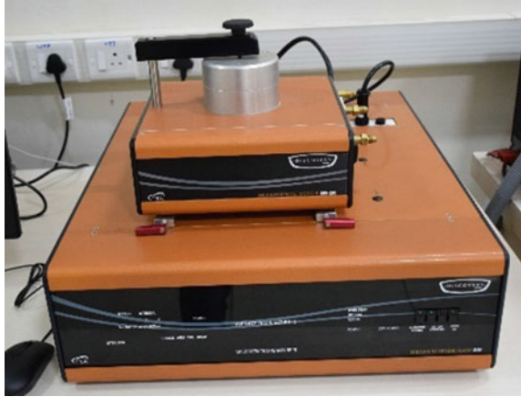
Fig. 6 Thermal conductivity measurement set-up (Make-TA, Model-Discovery Xenon Flash DXF 200)
