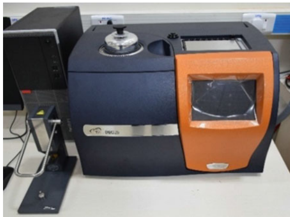
Fig. 5 Differential scanning calorimeter (Make-TA, Model-DSC-25)
