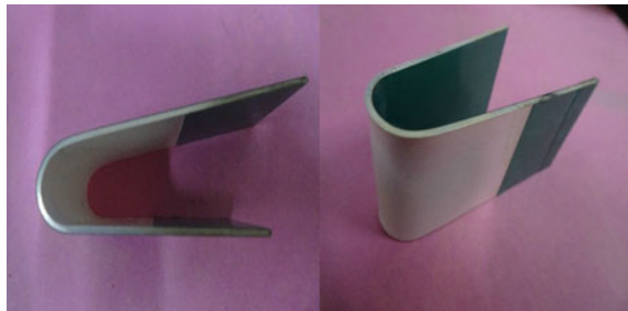
Fig. 7 Bend test (compressive side and tensile side)
