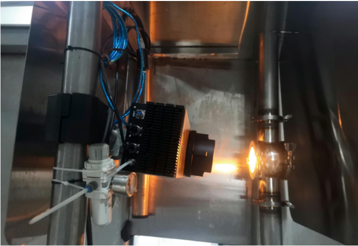
Fig. 7. On-line near infrared spectroscopy probe for monitoring chemical reaction process
