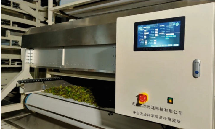
Fig. 4. On-line near infrared spectroscopy for detecting the quality of tea production process
