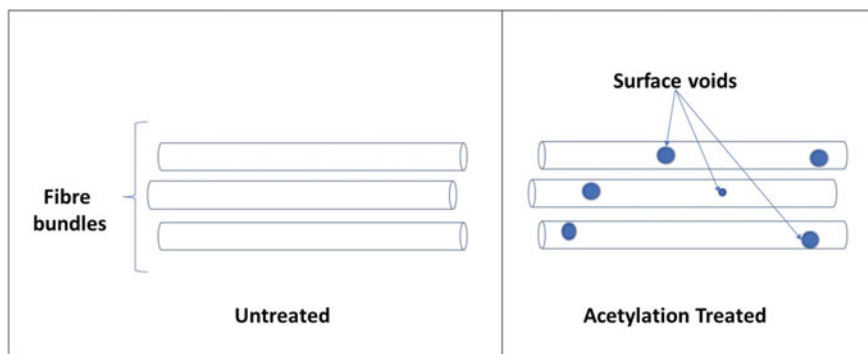
Fig. 10 Illustration of acetylation effect on the fibre surface
