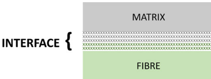
Fig. 15 Illustration of molecular entanglement at fibre–matrix interface
