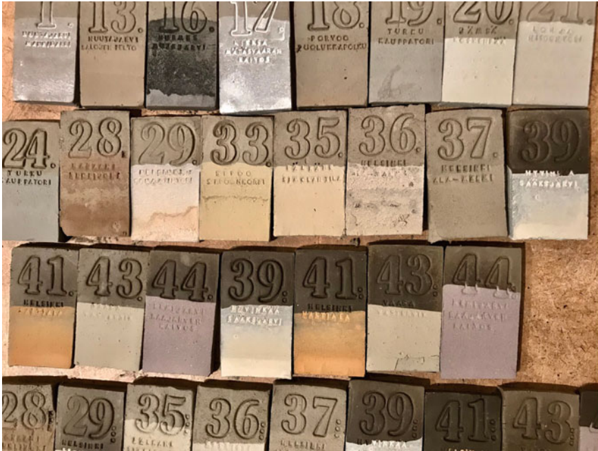
Fig. 4 Test pieces were made of Finnish earthenware clay, dipped in the processed soil samples from around Finland and left to dry before firing (Photo: Tzuyu Chen)
