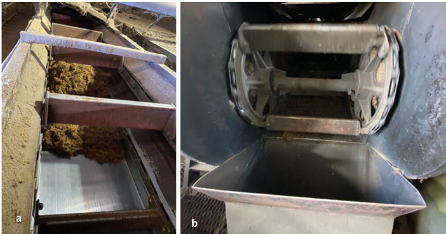
Fig. 3 a Scraper conveyor and b Wide openings under the conveyor to avoid blockage and bridging
