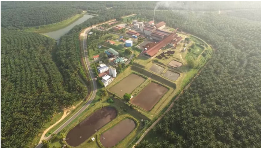
Fig. 25 A bird eye view of a POM with large area for POME treatment ponds
