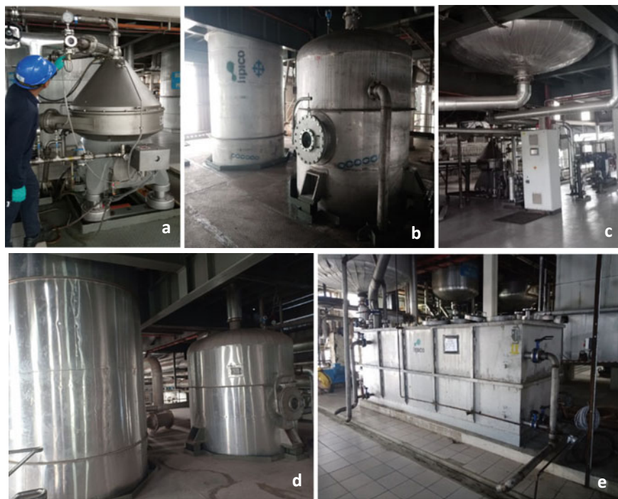
Fig. 14 CPO washing plant equipment, a Centrifuge; b–d Reaction vessels; e Settling tank
