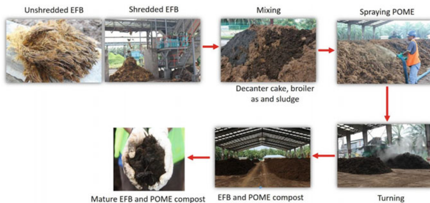
Fig. 8 Bioconversion of EFB and POME into organic fertiliser
