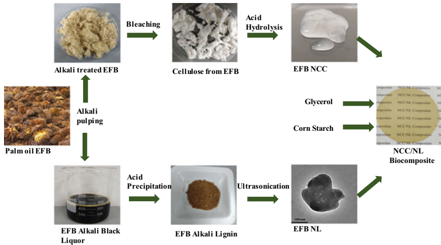
Fig. 1 The procedure to fabricate NL /NCC biocomposites
