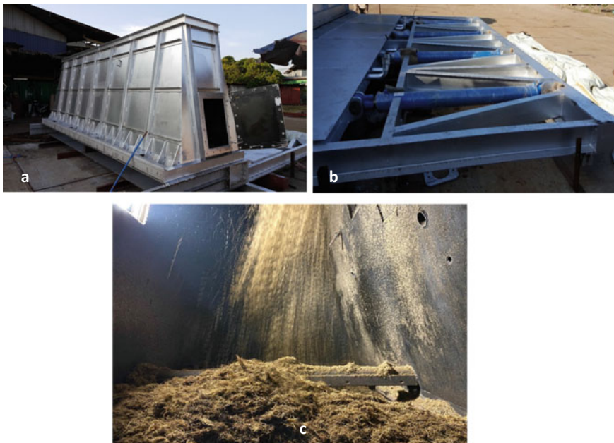
Fig. 4 Inverted “V” bin a Front view of the bin and service manhole, b Close up of the ram feeder located below the bin, and c EFB fiber filling the upside down V-bin
