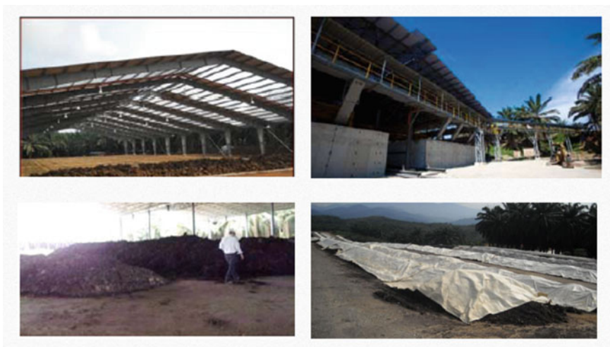
Fig. 16 Indoor composting process and outdoor composting process, turning EFB and POME into sellable compost
