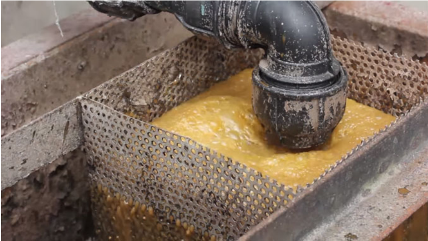
Fig. 24 A close-up picture of POME originated from the sterilization and extracting processes in a POM
