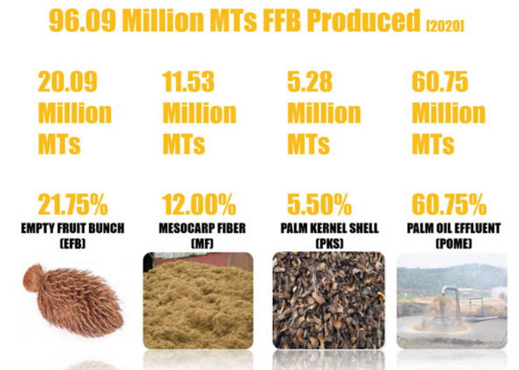
Fig. 13 Different types of biomasses generated from POM, calculative estimation to industrial best knowledge
