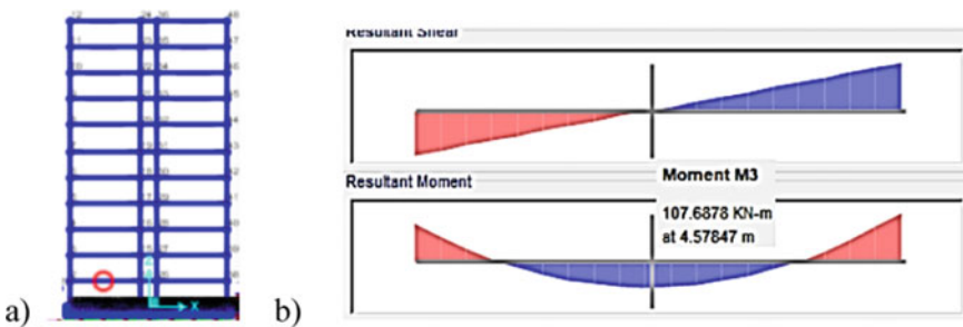
Fig. 4 Bending moment M = 107 kNm in the middle of the beam without CFRP. (a) Model of building to be studied; (b) Shear diagram and bending moment in the beam under consideration
