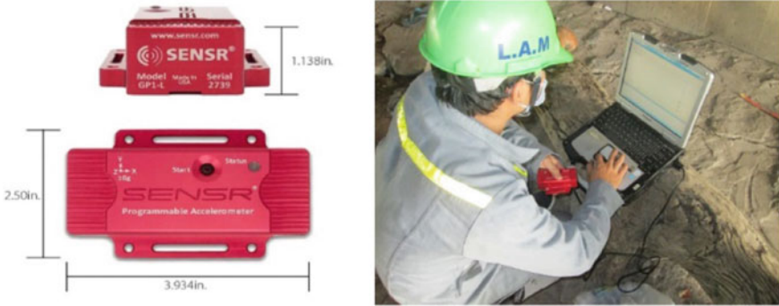
Fig. 4 Acceleration sensor (left) and data acquisition computer (right)
