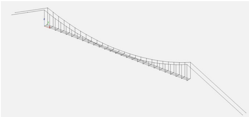
Fig. 4 FEM model of the bridge using MATLAB
