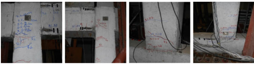
Fig. 3 Cracks in reinforced concrete frame model
