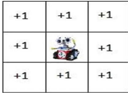
Fig. 1 A bot stuck due to equal reward in all the surrounding states [16]
