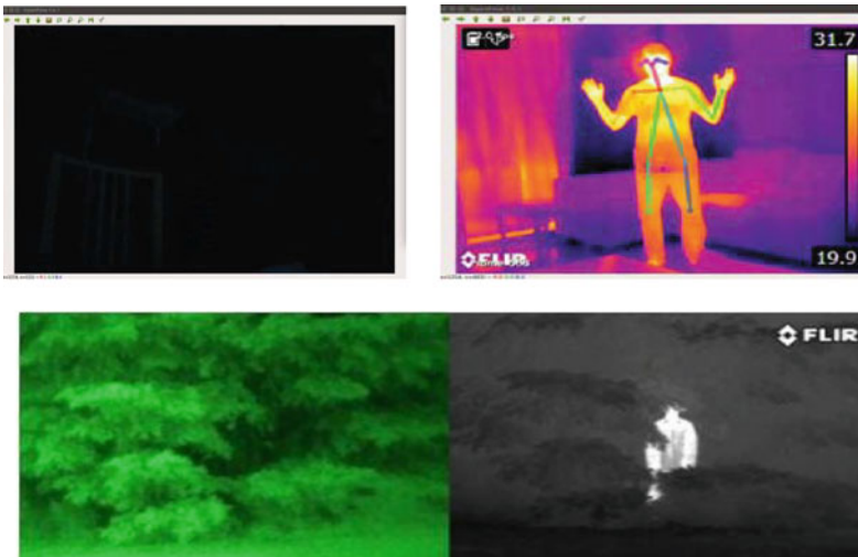
Fig. 2 a denotes image of an environment captured by a typical RGB camera and b denotes image of an environment captured by a thermal camera and c denotes image taken using night vision camera at the left and thermal camera at right
