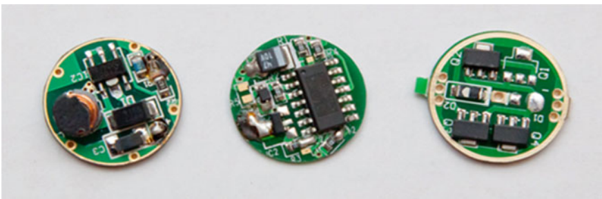
Fig. 5.27 Control circuits for regulation of illumination intensity and creation of light effects (image credit: Scilif s.r.o. company)
