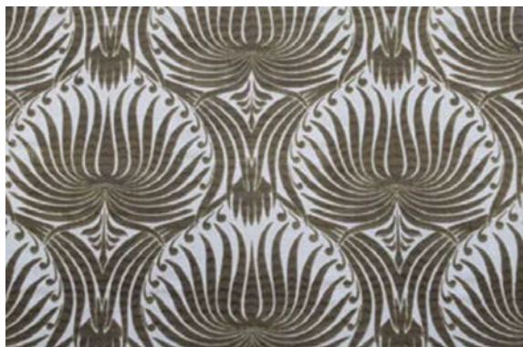
Fig. 1.10 Using of laser engraving for patterning of fabric
